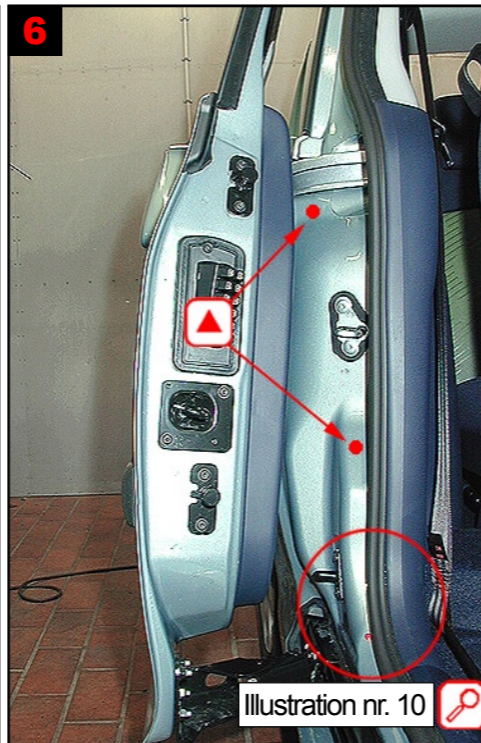
6 B-pillar and rear wing: Drill 2 holes for correct treatment. Panel: See fig 10.
