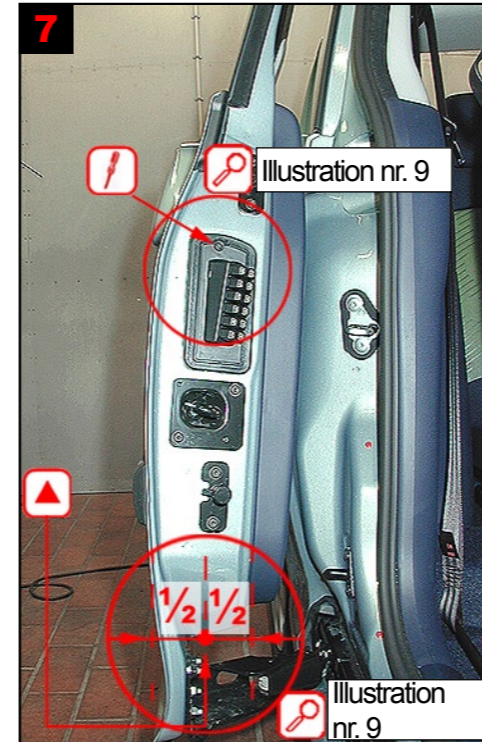
7 Sliding door: Remove door switch. Treat with lance. Fig. 9: Body frame: Treat via 3 drilled holes. Fig. 9:
