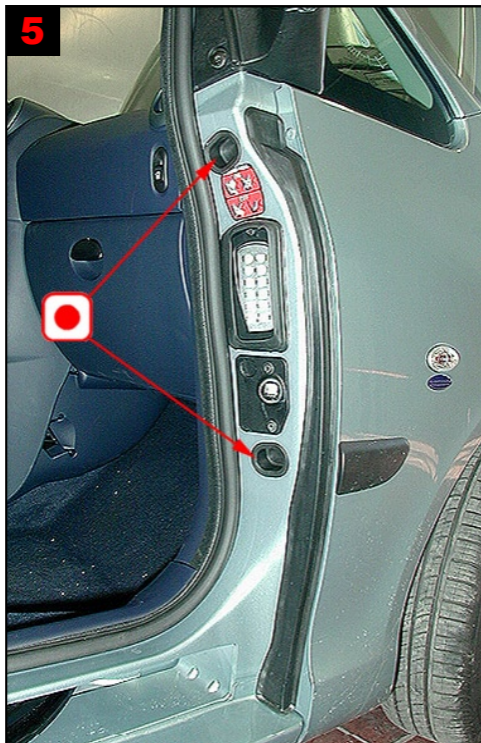
5 A-pillar: Treat via 2 existing plugged holes.
