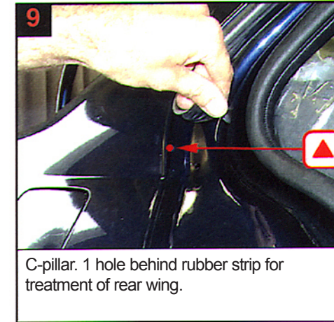
9 C-pillar. 1 hole behind rubber strip for treatment of rear wing.
