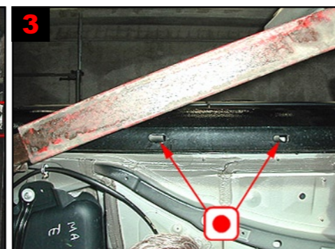
3 Panel: Treat via 2 existing plugged holes.
