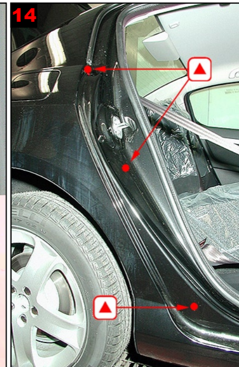
C-pillar and rear wing: Drill 2 holes - treat with lance. C-pillar/panel: Treat via 1 drilled hole.
