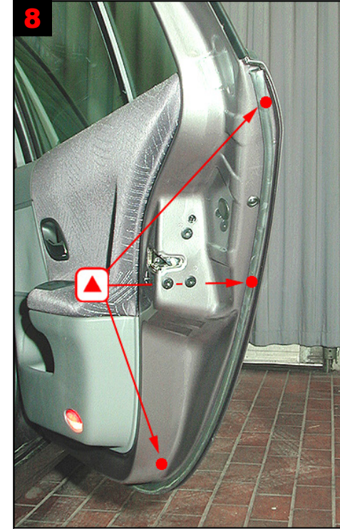
8 Rear door: Treat via 3 drilled holes. Uppermost drilling app. 5 cm down and behind rubber strip. Centre drilling, behind rubber strip and level with screws for locking device.
