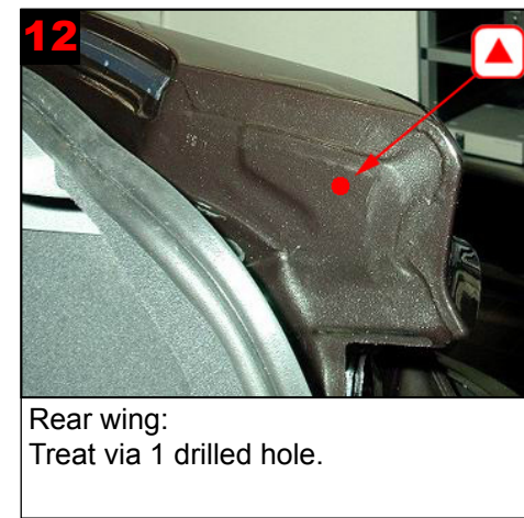
12 Rear wing: Treat via 1 drilled hole.
