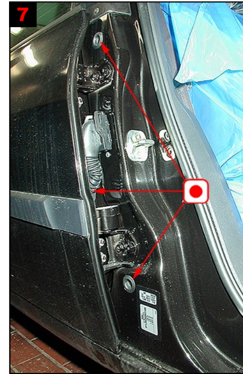
7 B-pillar/back door: Treatment of B-pillar via 2 existing plugged holes. Rear door: Treatment via grommet.
