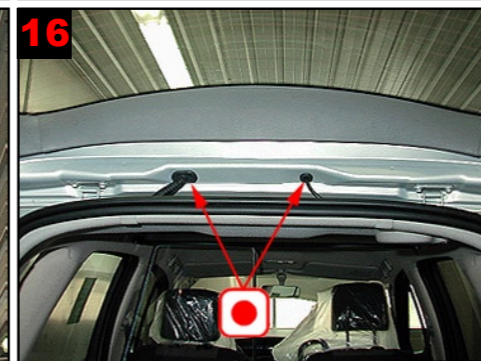
Tailgate by roof: Treatment via 2 plugged holes.
