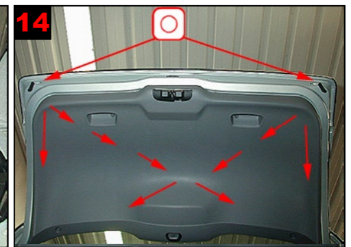
Tailgate by bumper: Via drain holes. Caution when advancing lance.
