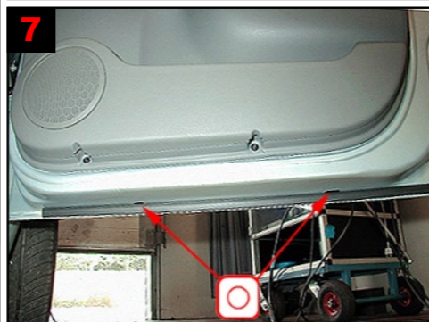
Front door bottom: Via drain holes. Caution when advancing lance.
