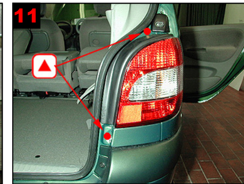
11 Rear wing/rear panel: Treat via 2 drilled holes.
