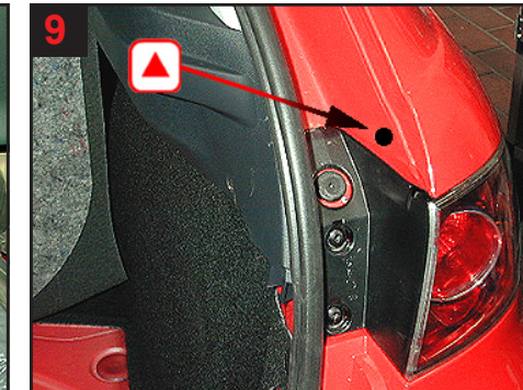
Rear wing: Treat via 1 drilled hole above tail light.
