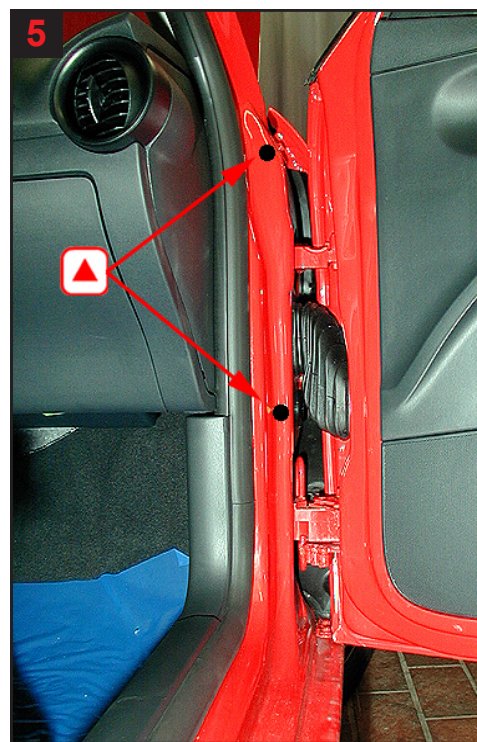
A-pillar: Treat via 2 drilled holes. Top drilling level with screw for wing. Lower drill hole: Drill level with plug.
