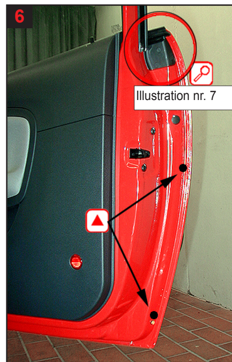
Door. See fig 7 for correct treatment of top member. Treat via 2 drilled holes. Top drilling level with screw for lock mounting.
