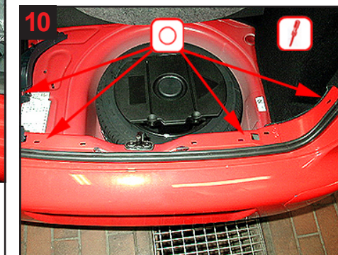
Rear panel: Remove plastic plate and side fittings. Treat via existing holes.
