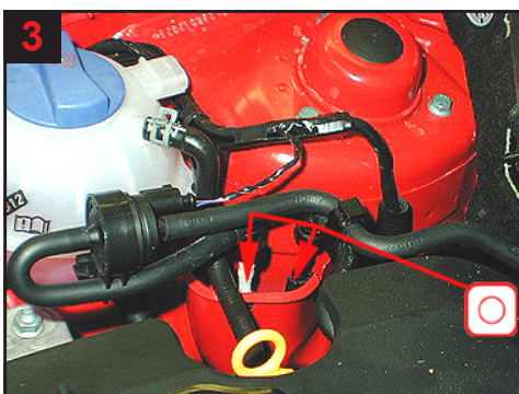
Engine compartment: Treat reinforcements via existing gap.
