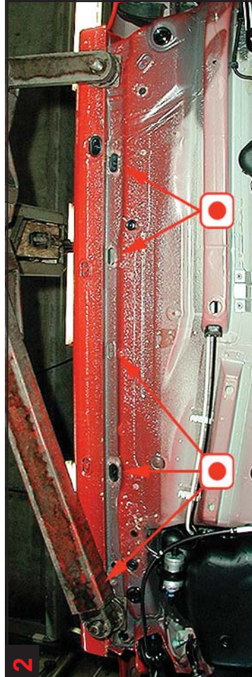
2 Panels: Treat via 4 existing plugs for treatment of inner panel and 4 existing plugs for treatment of outer panel.
