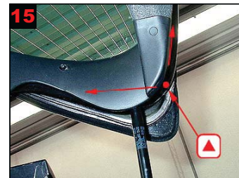
15 Tailgate side: Treat via 1 drilled hole each side.
