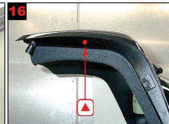
16 Tailgate side: Treat via 1 drilled hole each side. Tailgate:
