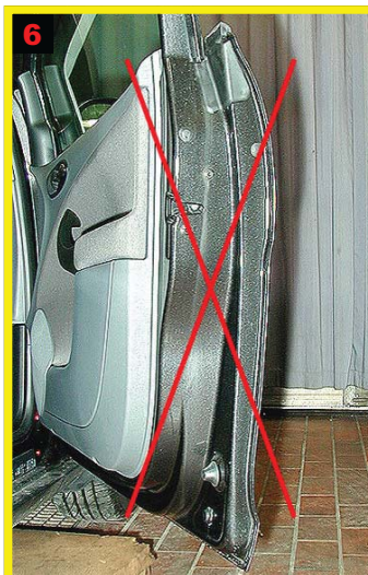
6 Front door: No treatment pressure sensor for AIRBAG.
