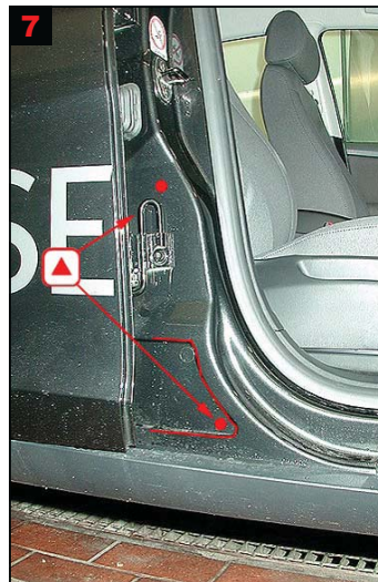
7 B-pillar: Drill 2 holes for correct treatment.
