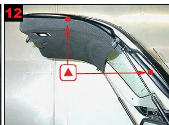
12 Tailgate side: Drill 2 holes for correct treatment.
