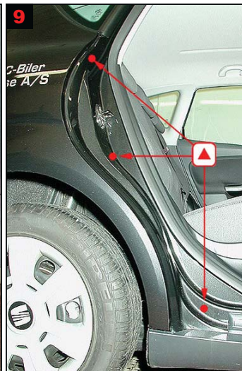
9 C-pillar: 3 drill holes for correct treatment.
