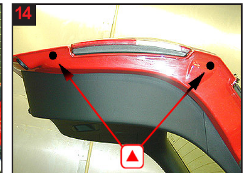
Tailgate by bumper: Drill 2 holes for treatment with lance.
