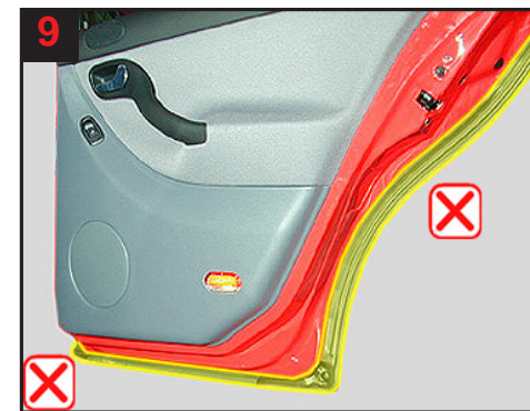
Rubber strips in general. Protect/cover as these are not resistant to oil (around drain holes).
