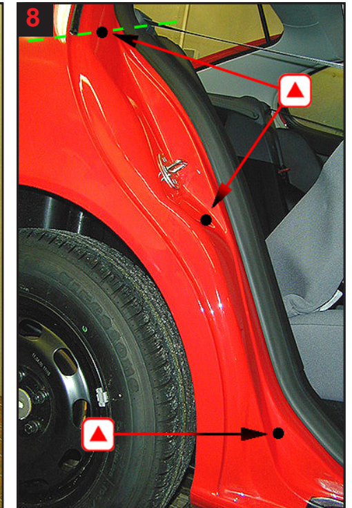
C-pillar: Treat via 3 drilled holes. Uppermost drill hole for part treatment of rear wing.
