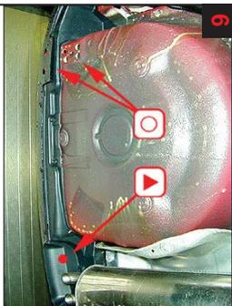
6 Rear panel and reinforcement. Drill 1 hole in plastic plate (left side) - remaining treatment via existing holes.
