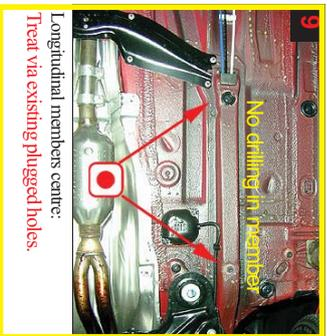
9 Longitudinal members centre: **No drilling in member!** Treat via existing plugged holes.
