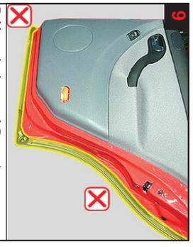
9 Rubber strips in general. Protect/cover as these are not resistant to oil (around drain holes).
