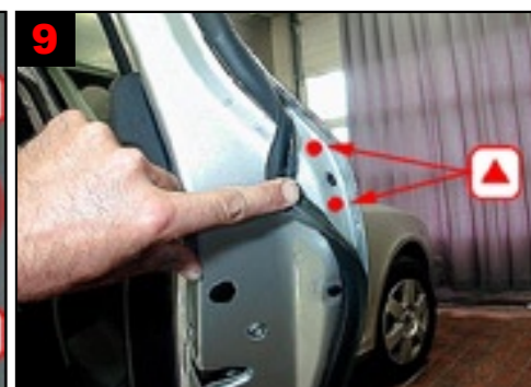
9 Rear door sectional view: Top member: Treat via 2 drilled holes. Flip rubber strip, drill behind it.
