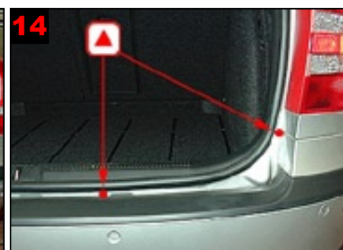
14 Fig: drilling at correct level.
