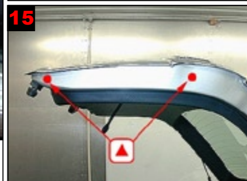
15 Tailgate side: Drill 2 holes for correct treatment (caution when advancing lance).
