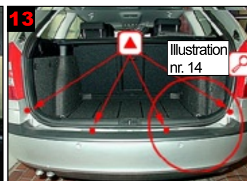
13 Rear panel: 4 drill holes for correct treatment. See fig 14 for drilling at correct level.
