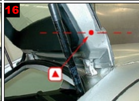
16 Tailgate side by roof: Treat via 1 drilled hole each side. Treatment with lance or flex hose.
