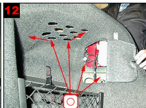
12 Rear wing from boot: Treatment via existing lug by tail light, treat with caution in all directions. Treat behind lining. Treat via existing holes. Caution around lining.
