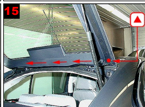
15 Tailgate side by roof: Treat via 1 drilled hole each side. Treatment with lance or flex hose.
