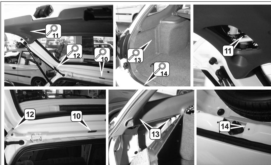
10. tailgate; front section; remove rubber sealing
