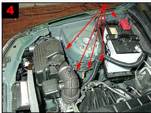
4 Engine compartment sectional view, right side: Reinforcement on spring strut. Treat via existing holes and gaps. Treat under battery and airfilter box and behind spring struts.
