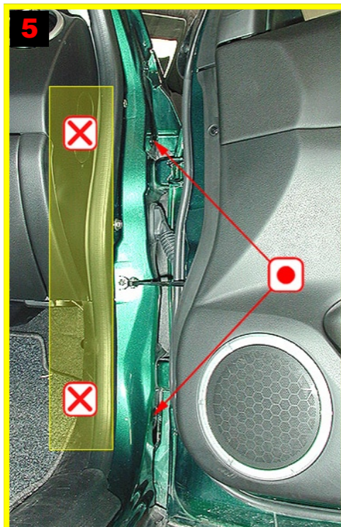
5 A-pillar: Treatment via 2 plugged holes. No spraying towards cabin.
