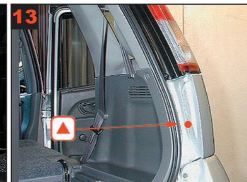
13 Rear wing: Treatment via 1 drill hole below tail light.
