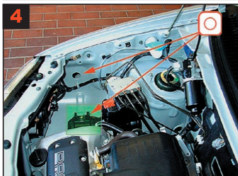
4 Engine compartment - sectional view: Treat engine suspension via existing hole. Treat front wing via existing holes.
