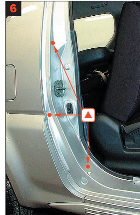
6 B-pillar and rear wing: 3 drill holes for correct treatment.
