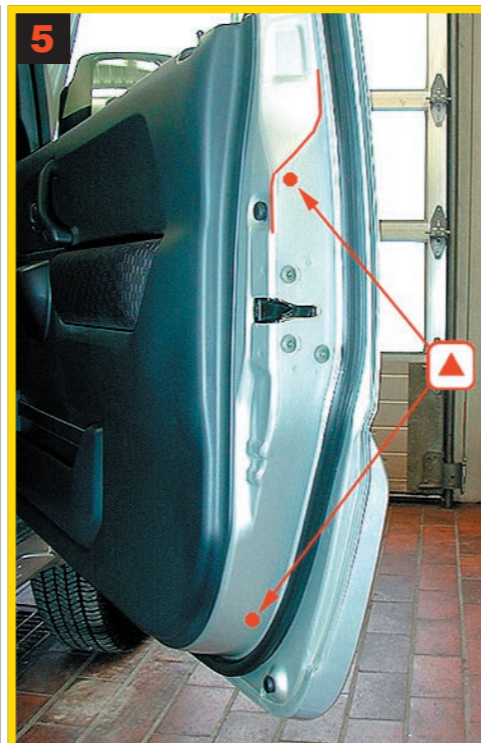
5 Front door: Drill 2 holes for correct treatment. Caution when advancing lance.
