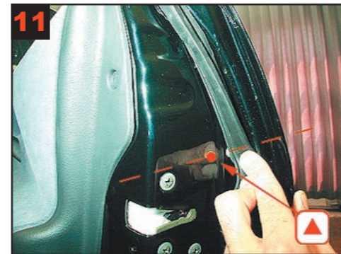
11 Rear door sectional view: Drill hole level with clips for rubber strip.
