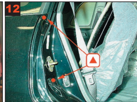
12 C-pillar: Treat via 2 drilled holes.
