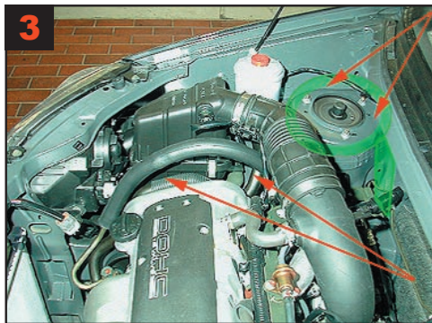
3 Engine compartment sectional view, right side: Treat under airfilter box and behind spring struts.
