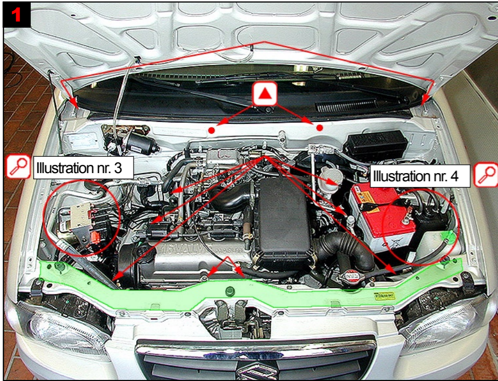
1 Engine compartment: Cowl: Treat via 2 drilled holes. Caution when treating from sides. Treatment on top of longitudinal members, behind spring struts, under battery and fuse box and treatment of reinforcement for engine suspension. Treatment of locking plate via existing holes and up under. See fig 3 and 4 for correct treatment.
