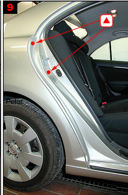
C-pillar: Treat via 2 drilled holes.
