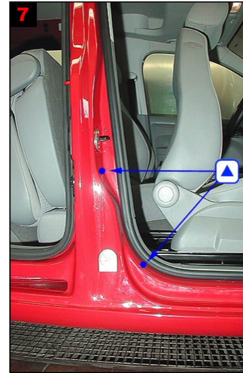
7 B-pillar and rear wing: Treat via 2 holes for correct treatment.
