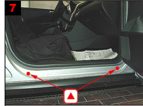
Panel: Treat via 2 drilled holes.
