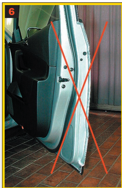
Front door: No treatment pressure sensor for AIRBAG.
