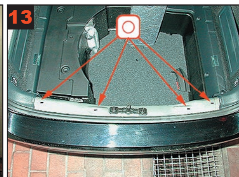
Rear panel: Remove plastic plate and treat via existing holes.
