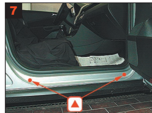
Panel: Treat via 2 drilled holes.
