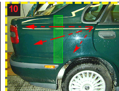
10 Rear wing. A baffle cushion is fitted into the rear wing, caution is needed in passing it.
