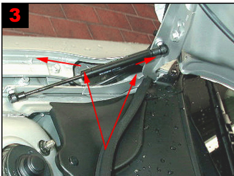
Engine compartment/front wing: Treatment via existing gap by hinges for bonnet lid.
