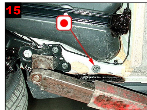
15 Longitudinal member before wheel arch rear: Treat via existing plugged hole.
