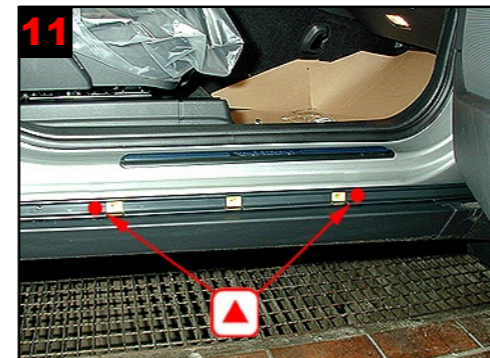
11 Panel - front door: Fig: drilling at correct level.
