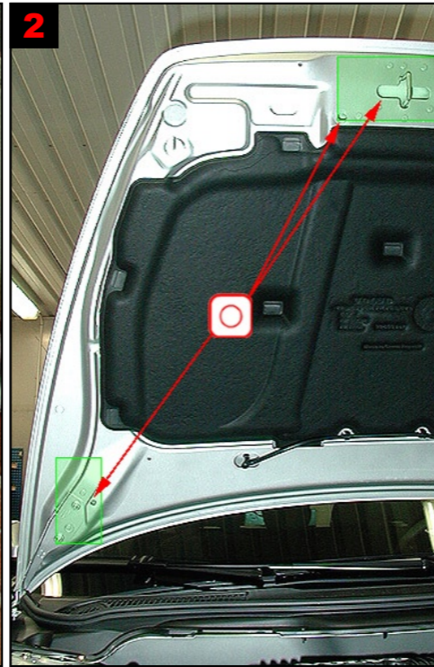
2 Bonnet lid (plastmaterial): Treatment of reinforcement via existing holes.
