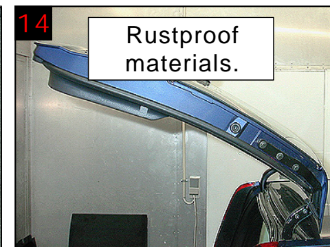
14 Tailgate: No treatment, rustproof materials.
